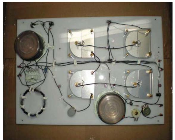
Inside: Note the bundle of wire at lower left - the broadcast antenna that creates the field sensed on the rub plate.
