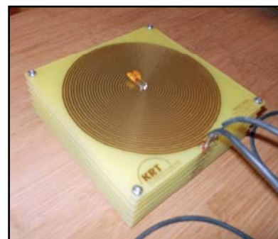
Six stacked plates turn individual antennas into an antenna array.
