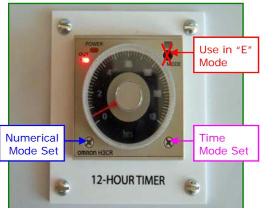
For example, changing the numerical mode on the timer shown in the photo would cause it to operate as a 1.2 Hour Timer, a 3 Hour Timer, a 12 Hour Timer, or a 30 Hour Timer.
