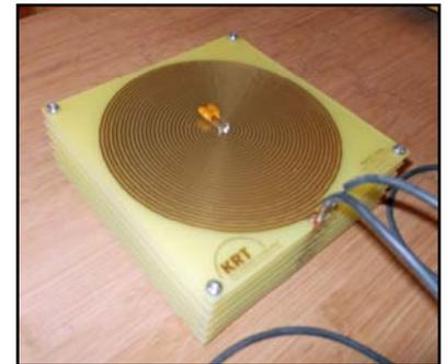
Six stacked plates turn individual antennas into an antenna array.
