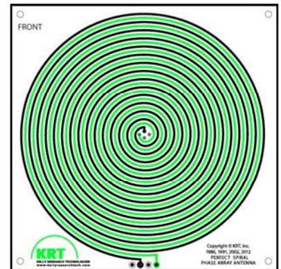
The signal rotates clockwise on the black path from edge to center, then counterclockwise on the green path from center back to the edge.
