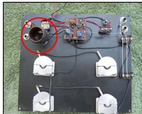
The air-core induction coil in a vintage Kelly Personal Instrument. To the right is an early solid-state amplifier board.
