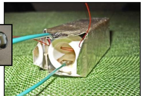
The induction coil and silver resonating strip are visible inside the Sephorah. The green wires tie the strip and the Sephorah to the “Signal In” connector.
