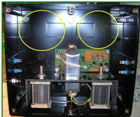
Visible pre-wiring, the single bank of plate capacitor tuners, silver Sephorah radio coil and solid state amplifier. Yellow circles show approx. location of input and output wells.
