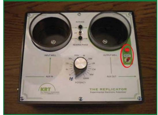
**Note:** To avoid burning out the relay that controls the clearing circuit, do not activate the instrument reset for longer than 2 seconds at a time.
