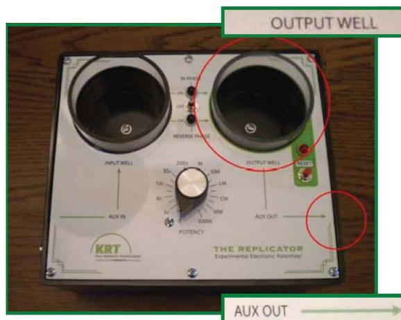
C. **Activate the Replicator by setting the phase mode switch** to "In Phase" or "Reverse Phase". A green indicator lamp will illuminate to show the mode that has been selected.
