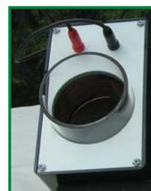
B. **Direct input from soil, plant or other probes** may be achieved by plugging any probes equipped with banana jack connectors into the gray "Aux In" jacks found on the left side of the Replicator.
