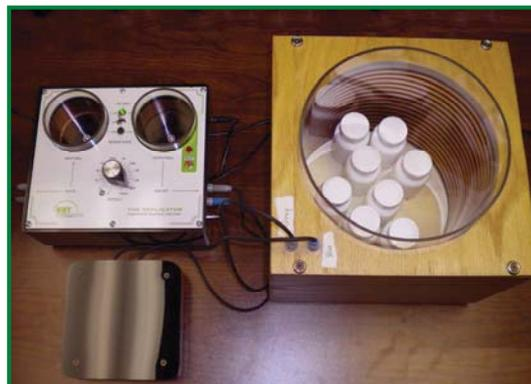
F. **Replicator output** may also be routed directly to either probes, external antenna or other devices through either the gray "Aux Out" jacks or the BNC connector found on the right side of the device. A pair of stacking jack connectors may be employed to allow simultaneous connection of probes and the reaction plate/antenna.
