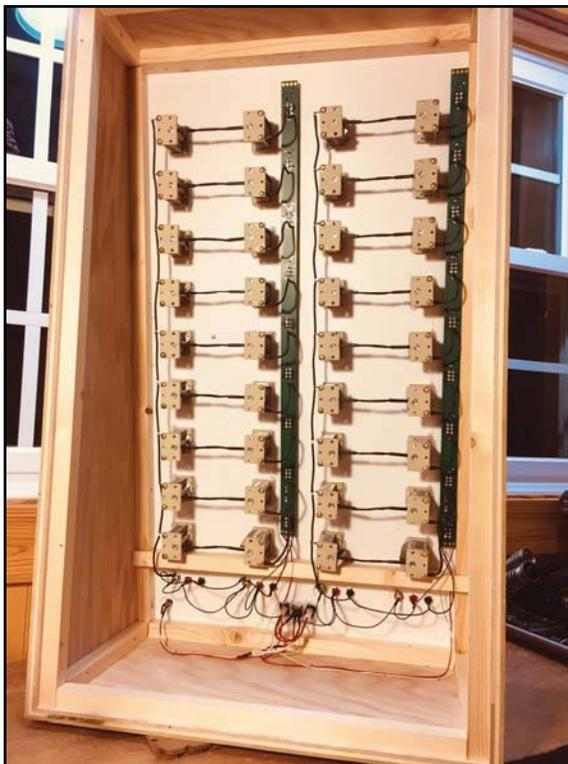
Variable Plate Capacitors in a Super Tuning Station, each with 19 Fixed and Rotating Tuning Plates for Maximum Resonance and Accuracy
