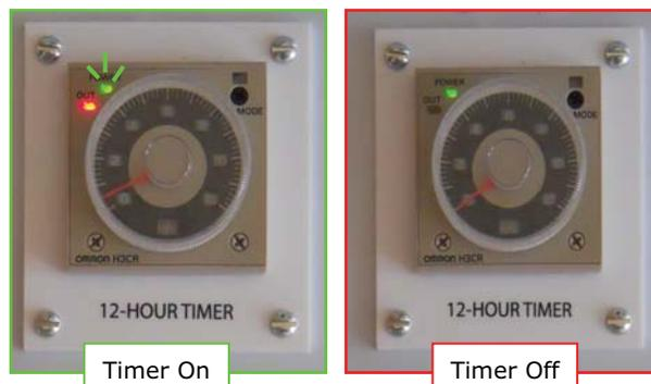
**Timer On:** When the timer is active and on the lamp marked OUT will be lit steady red and the lamp marked POWER will be lit green and flashing. At this time the flow of power to the amplifier is being controlled by the timer.
